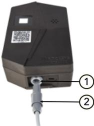
1. Insert the plug into the corresponding socket of the Watchdog.
